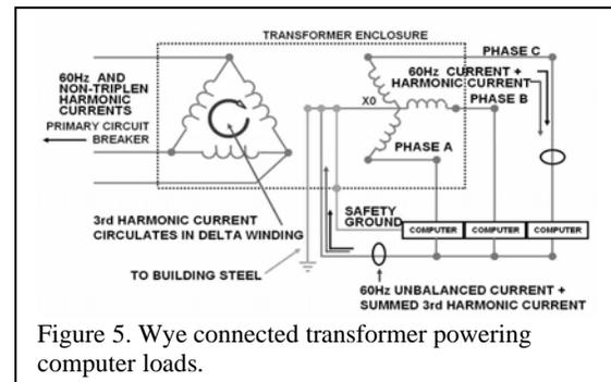
Figure 5. Wye connected transformer powering computer loads.
