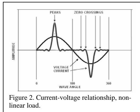
Figure 2. Current-voltage relationship, non-linear load.
