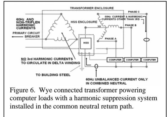
Figure 6. Wye connected transformer powering computer loads with a harmonic suppression system installed in the common neutral return path.
