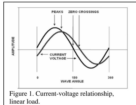
Figure 1. Current-voltage relationship, linear load.
